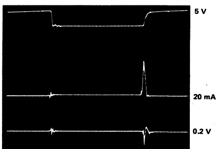
j) SN74ALS00A load: C_L = 50 \text{ pF}
